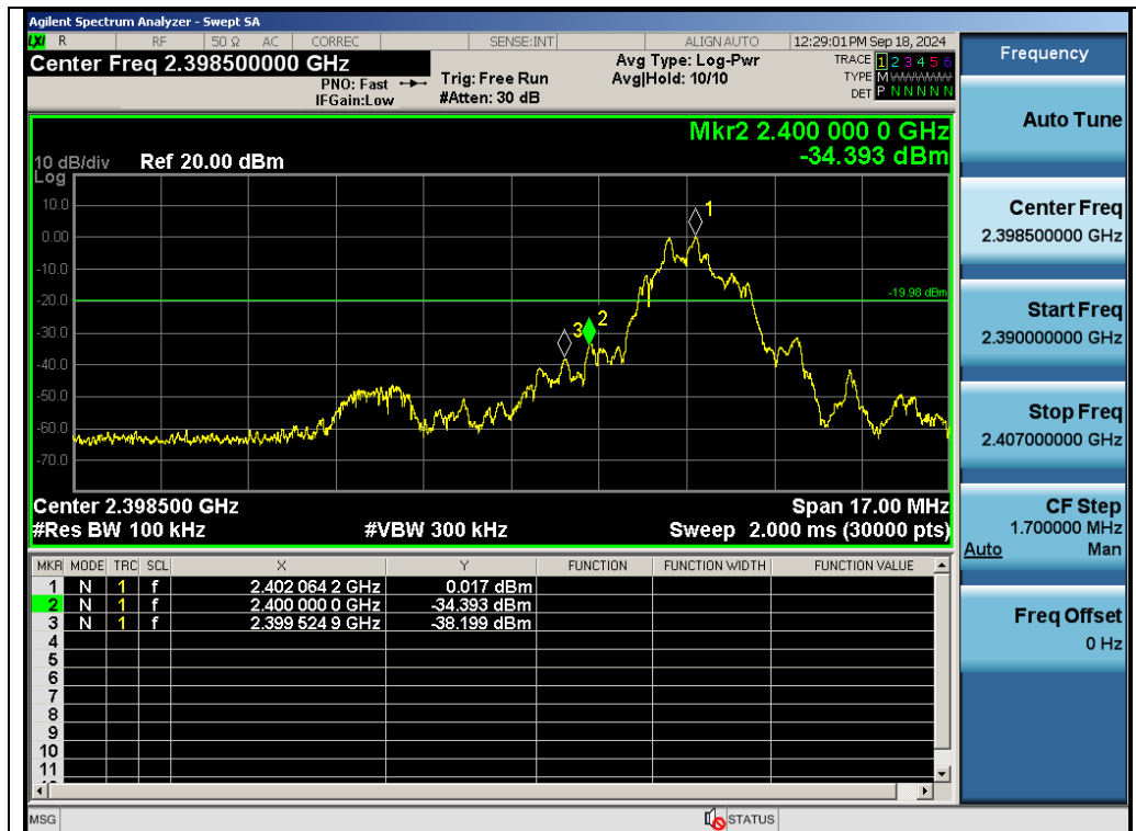
Test_Graph_LE2M_ANT1_2402_2Mbps_Lower Band Edge Emissions
