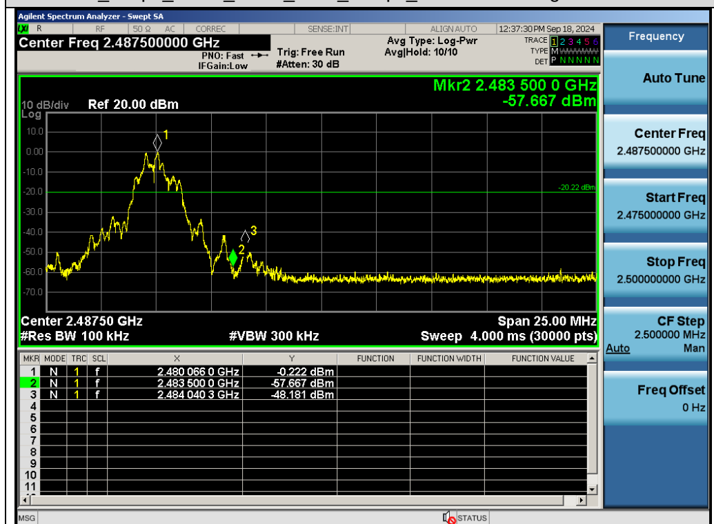
Test_Graph_LE2M_ANT1_2480_2Mbps_Higher Band Edge Emissions
