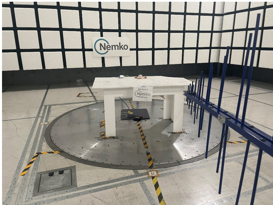
Figure 8.1-6: Radiated emissions setup photo, front – above 30 MHz
