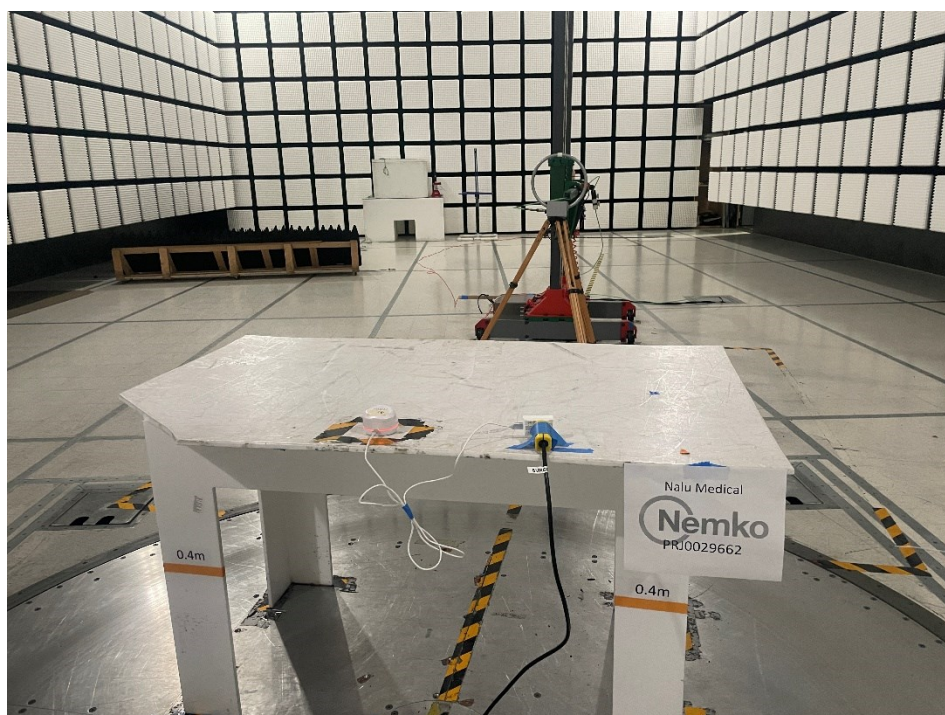
Figure 8.1-5: Radiated emissions setup photo, back – below 30 MHz
