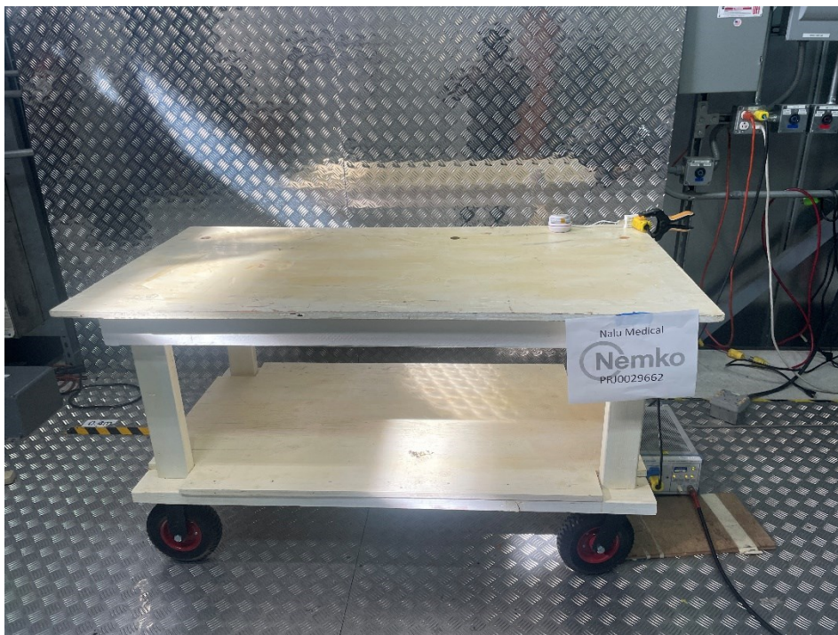
Figure 8.2-2: Conducted emissions from AC mains power ports setup photo
