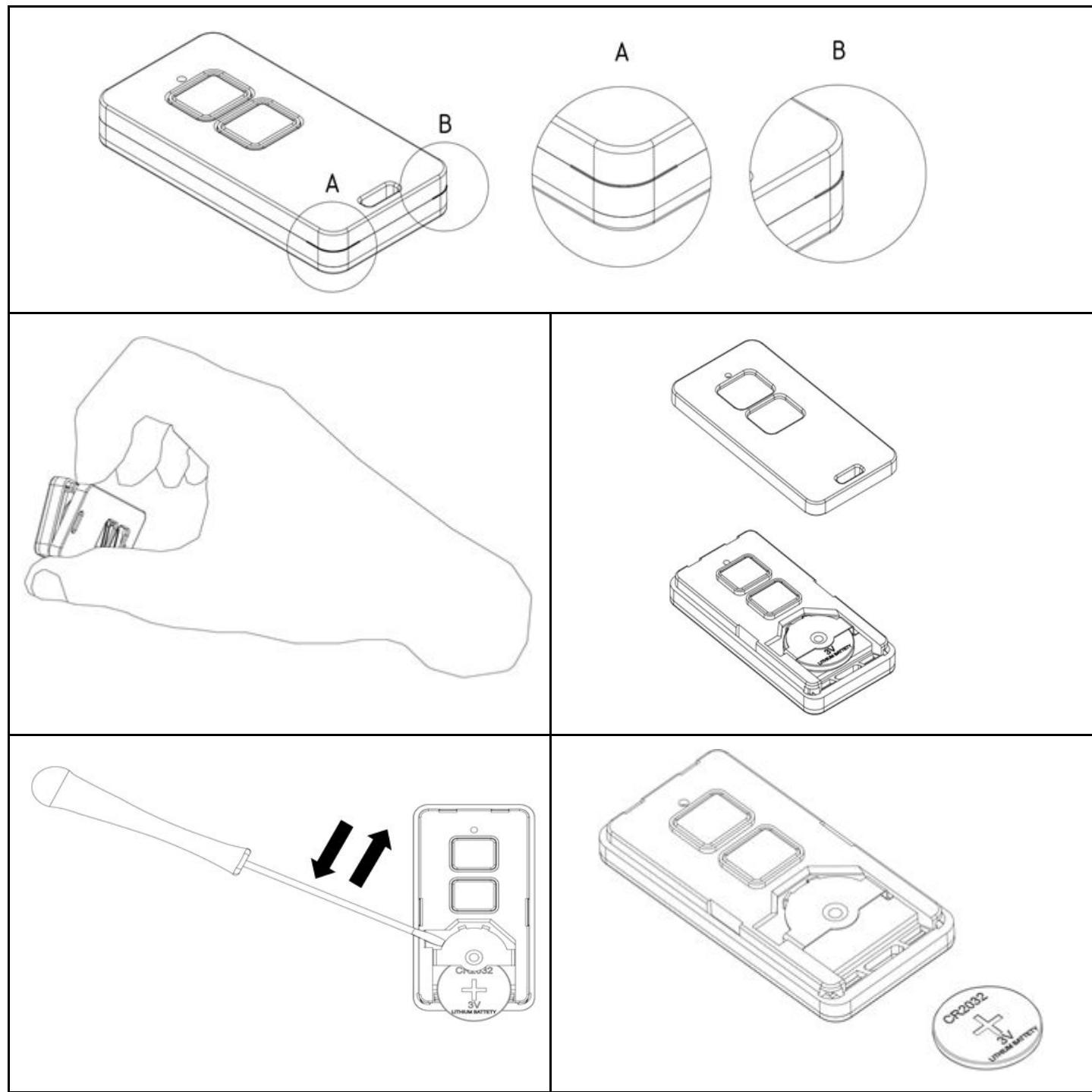
**After the replacement, discard the battery in an appropriate place.**
