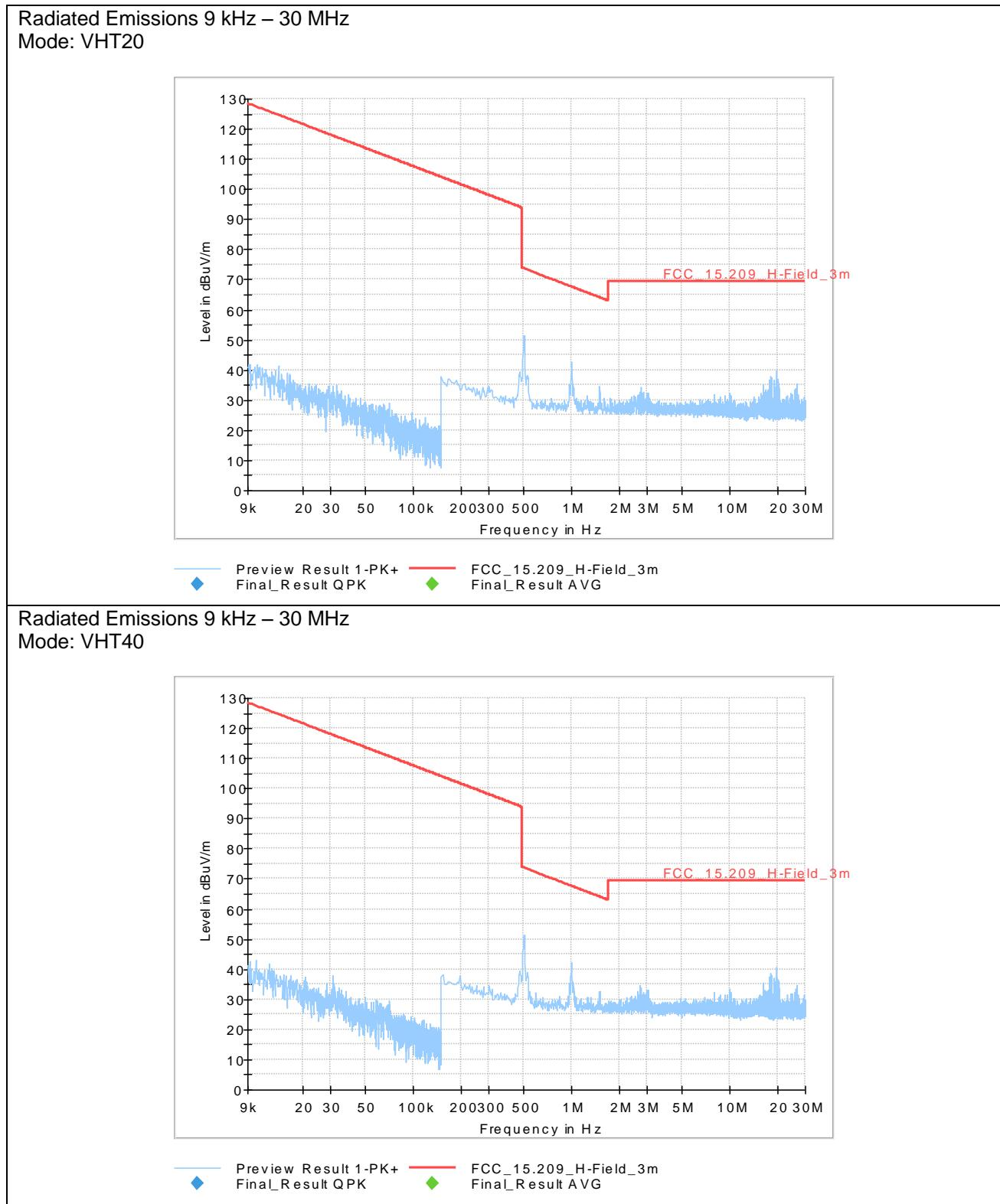
Test of Wireless Router type Bitdefender BOX 2 Smart Home Cybersecurity Hub
