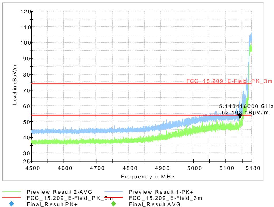
Test of Wireless Router type Bitdefender BOX 2 Smart Home Cybersecurity Hub
