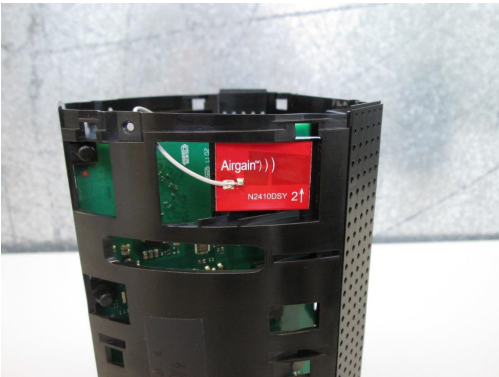
Photo A2-8: Placement of Antenna #2
