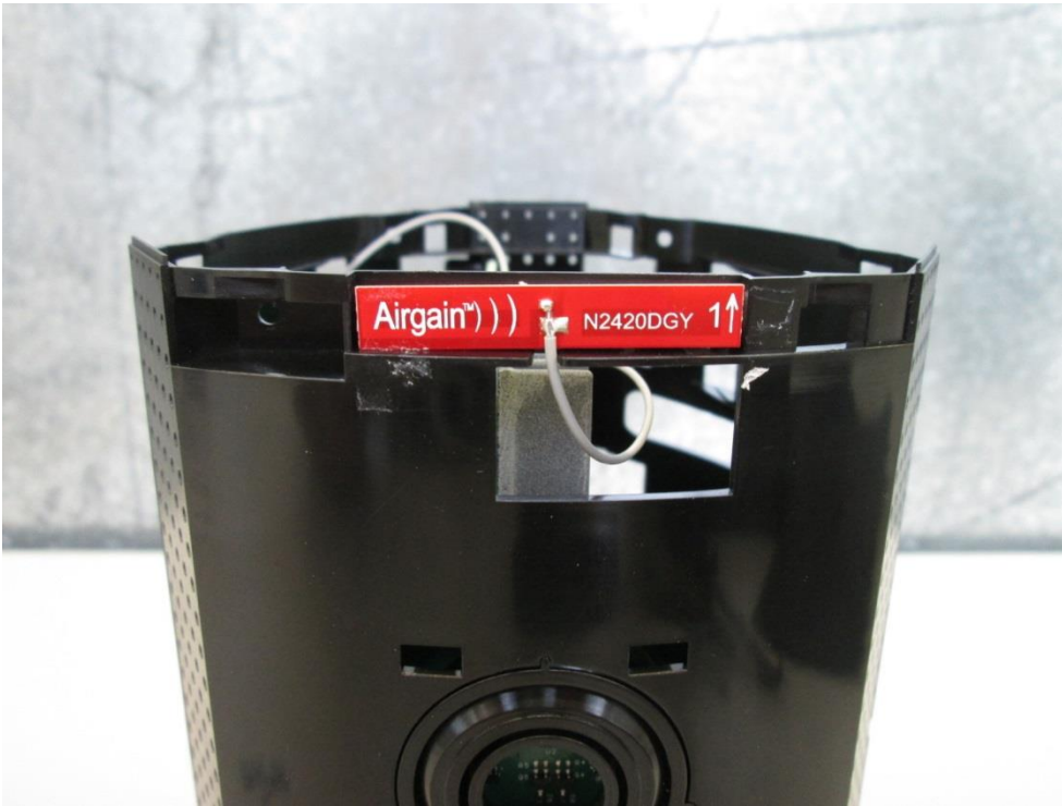
Photo A2-7: Placement of Antenna #1
