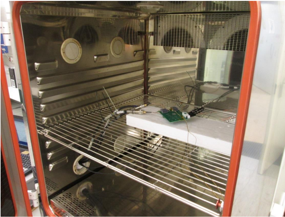
Photo A1-9: Frequency stability measurement in the temperature chamber
