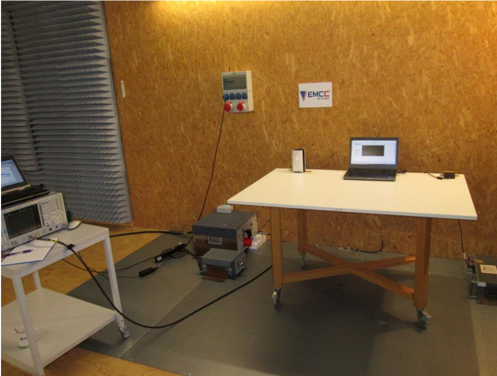
Photo A1-1: AC powerline conducted emissions measurement
