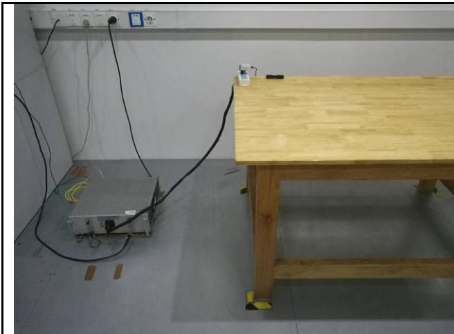
Conducted Emissions Test Setup Front View
