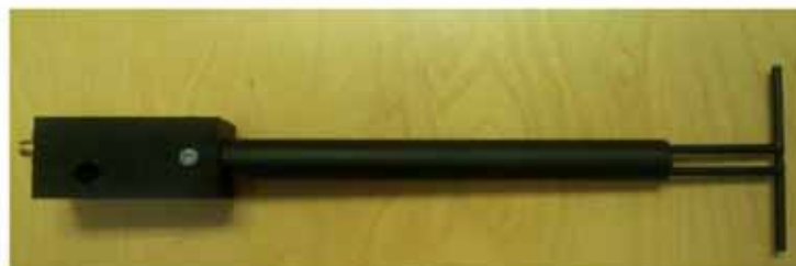
Figure 1 – MVG COMOSAR Validation Dipole
