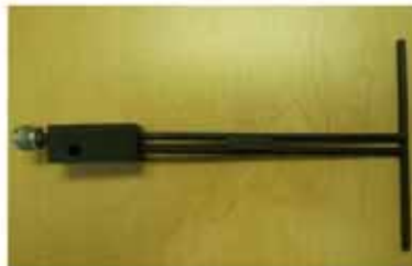
Figure 1 – MVG COMOSAR Validation Dipole
