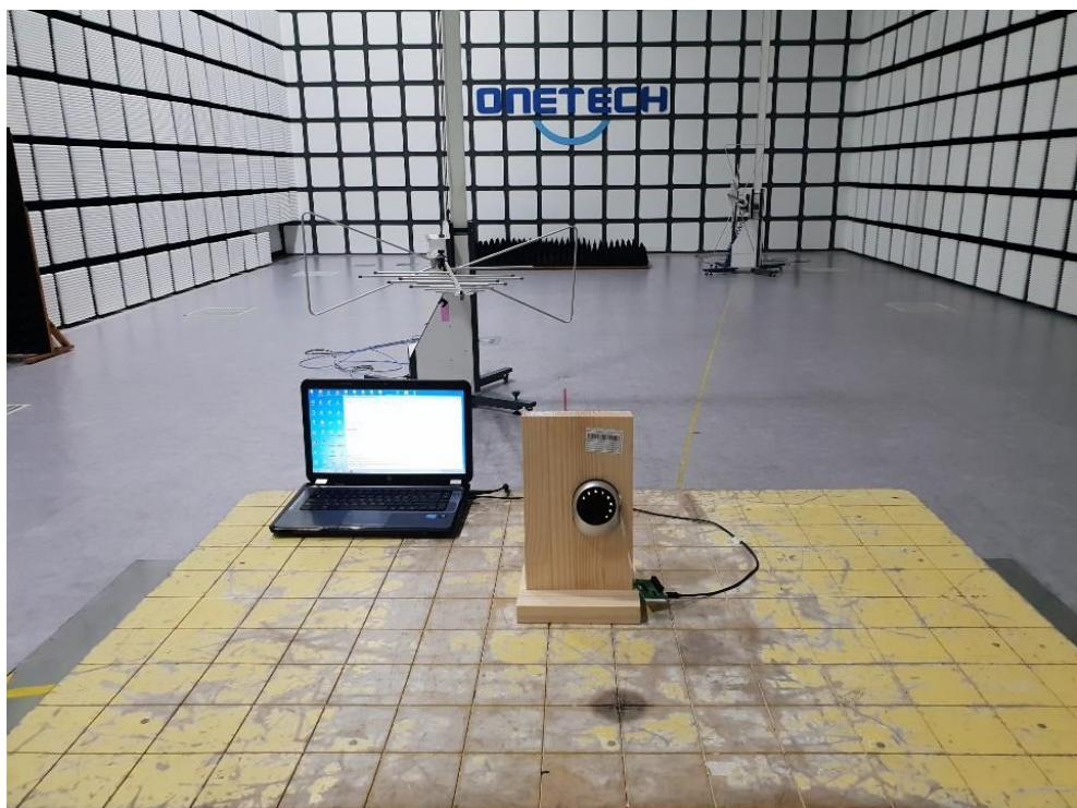
**- Radiated Emission Test for LE (Above 1 GHz)**
