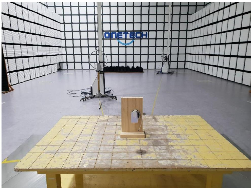
**- Radiated Emission Test for NFC (30 MHz ~ 1 GHz)**
