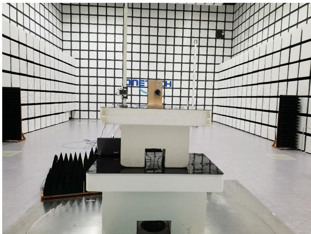
**- Radiated Emission Test for NFC (9 kHz ~ 30 MHz)**
