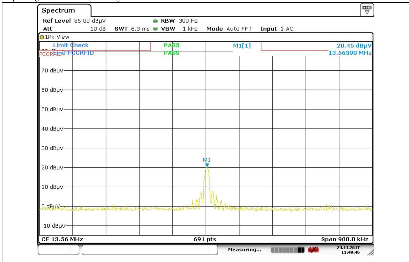
cc. to above test data, the field strength level of 13.563 9 MHz is 20.45 dBuV/m and the worst limit subject to 15.225 (b) and (c) is 80.5 dBuV/m, so the EUT meets the requirement.
