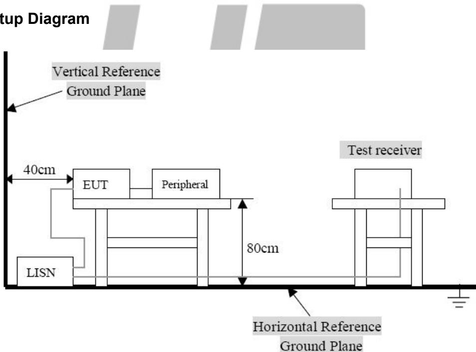
Remark: The EUT was connected to a 120 VAC/ 60Hz power source.
