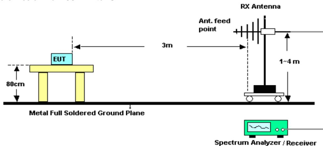
For radiated emission from above1GHz
