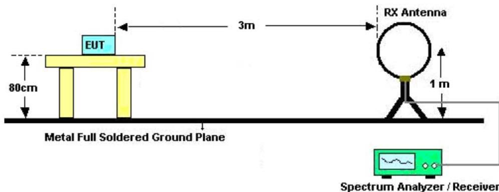
For radiated emission from 30MHz to1GHz
