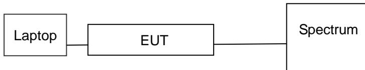
Note: 1. The EUT was powered using the standard Lab DC Power Supply for the testing to be in continuously transmitting mode and the transmit duty cycle is not less than 98%.
