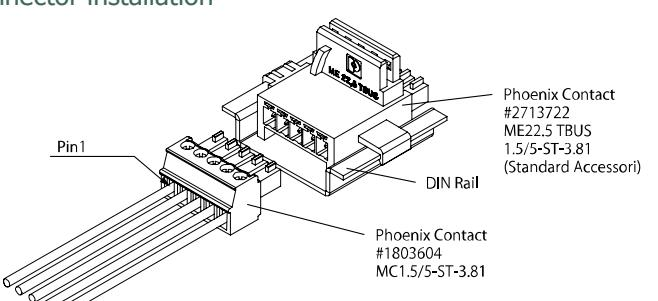
Attach the bus connector #2713722 to the fixed DIN rail, and then mount the AMG3002 after wiring the cables.
