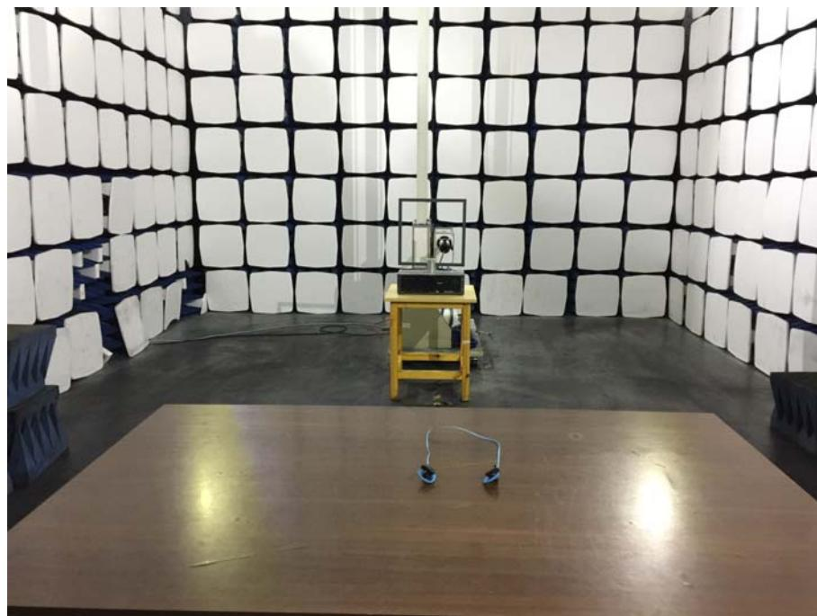
**Radiation Emission Test Setup (30MHz to 1GHz)**
