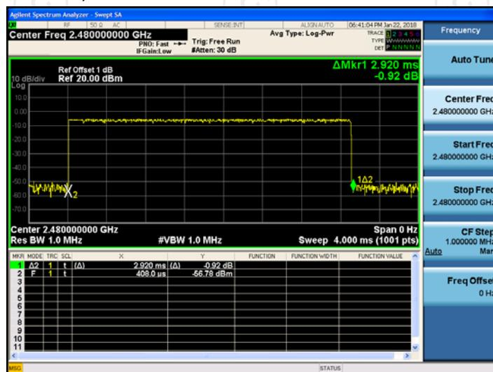
2DH5 on time (Count Pulses) Plot on Channel 78
