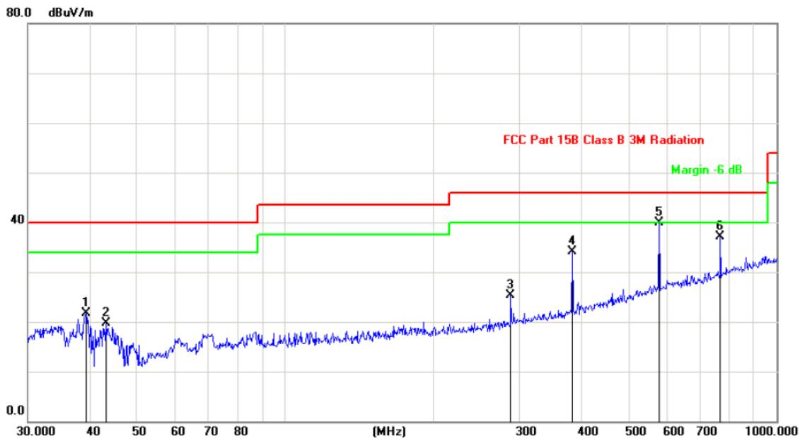
Site: FCC Part 15B Class B 3M Radiation      Polarization: Vertical      Temperature: 25
