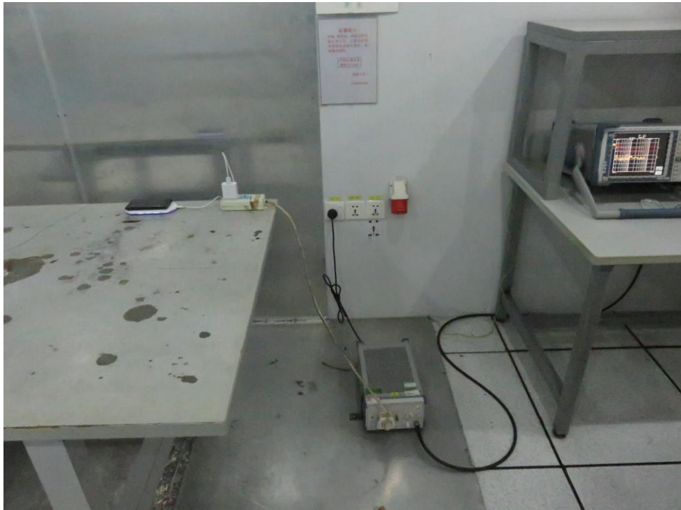
Photo of Conducted Emission Measurement
