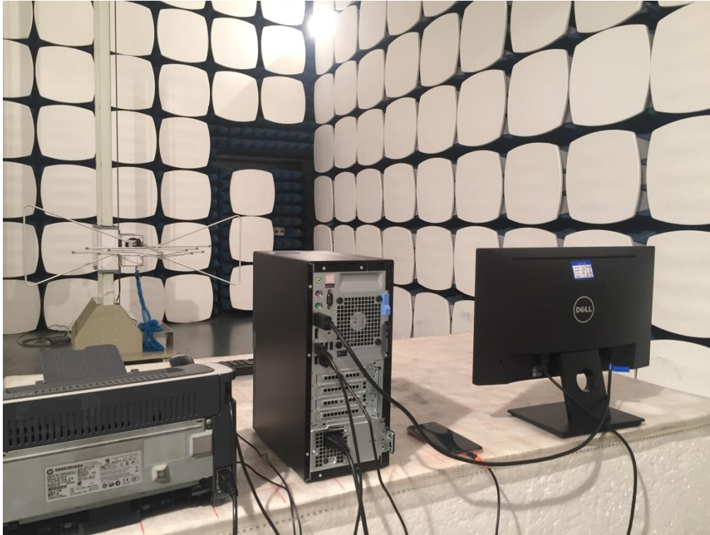
Radiated Emission Below 1GHz
