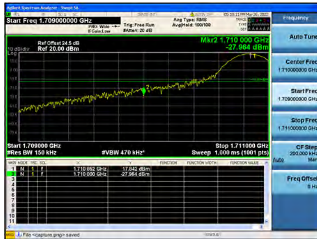
Band66 / 15MHz / High CH / QPSK / 1 RB
