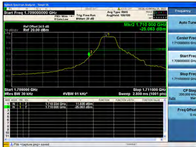
Band66 / 1.4MHz / High CH / QPSK / 1 RB
