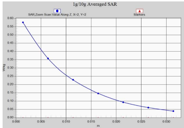
Fig.A.1- 4 Z-Scan at power reference point (PCS1900) AP OFF
