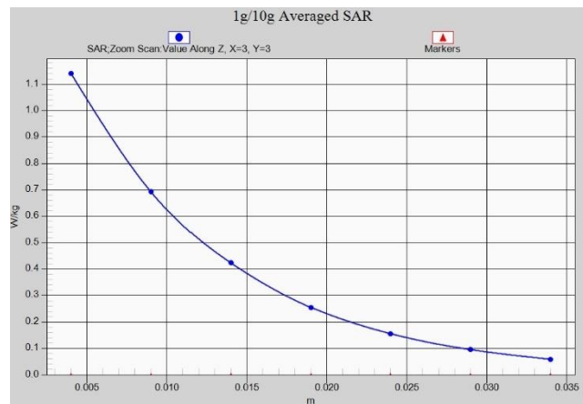
Fig. 1-4 Z-Scan at power reference point (PCS1900)
