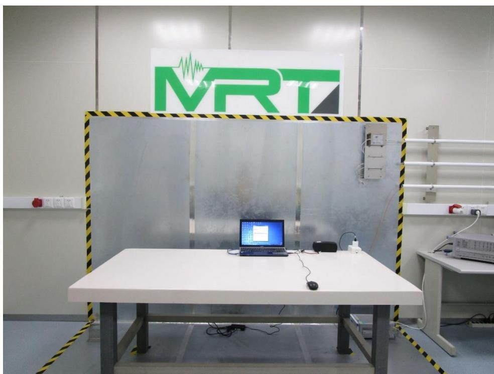
**Test Mode 1****Description: Back View of Conducted Emission Test Setup**
