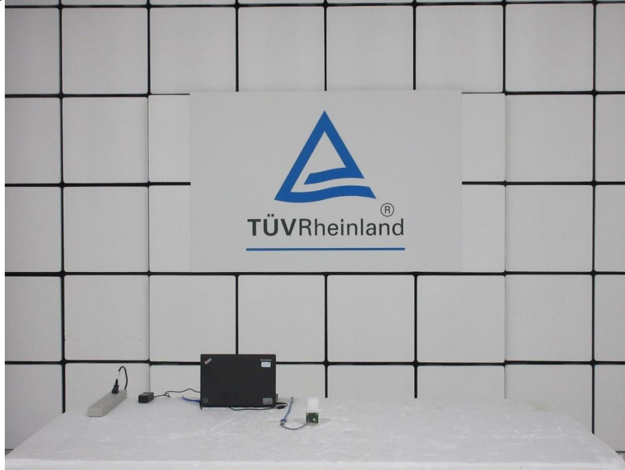
Photograph 1: Test Setup for Spurious Emissions (Front View 1)
