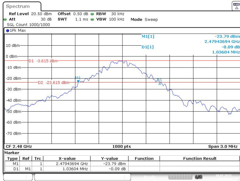
**FCC §15.247(a) (1) (iii)-QUANTITY OF HOPPING CHANNEL TEST****Applicable Standard**
