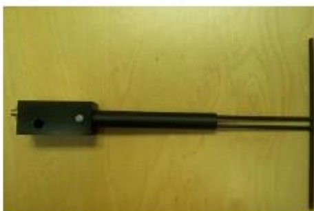
Figure 1 – MVG COMOSAR Validation Dipole
