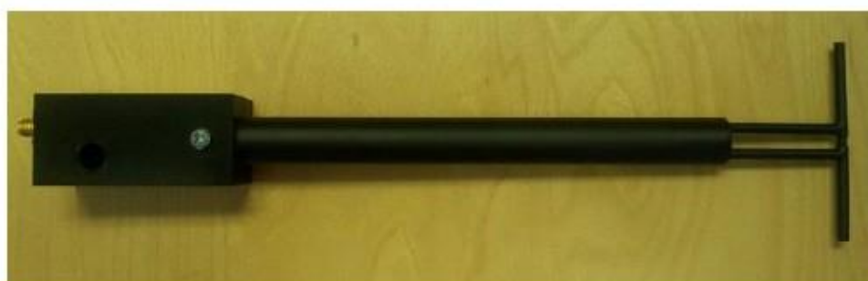
Figure 1 – MVG COMOSAR Validation Dipole
