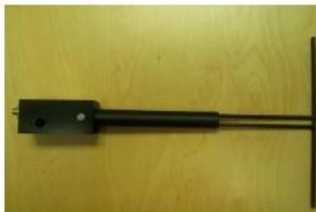
Figure 1 – MVG COMOSAR Validation Dipole
