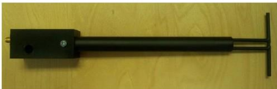
Figure 1 – MVG COMOSAR Validation Dipole
