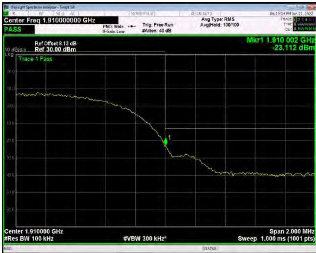
HSUPA Band2 Subtest3 Channel=9262 Band2 Normal
