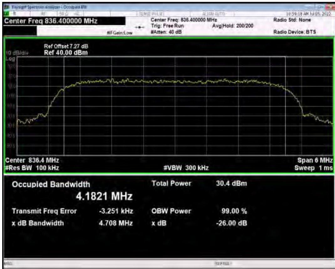
HSUPA Band5 Subtest1 Channel=4233 Band5 Normal
