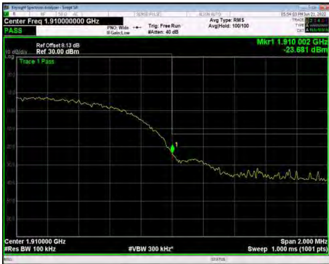
HSDPA Band2 Subtest3 Channel=9262 Band2 Normal
