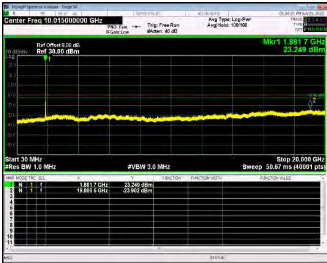
HSDPA Band2 Subtest1 Channel=9538 Band2 Normal
