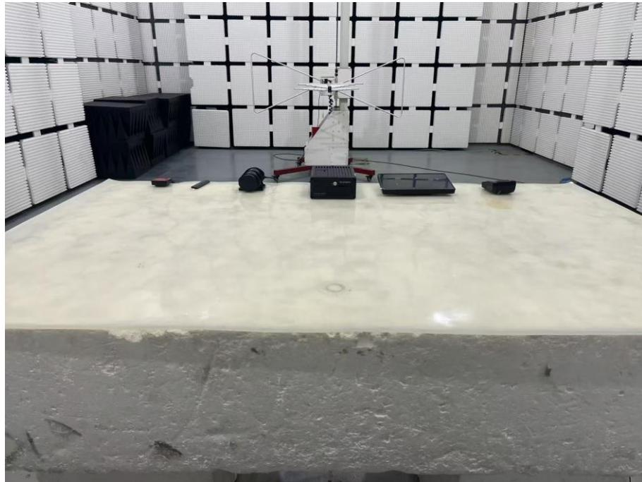
**Set-up for Radiated Emission (RE), Above 1GHz**
