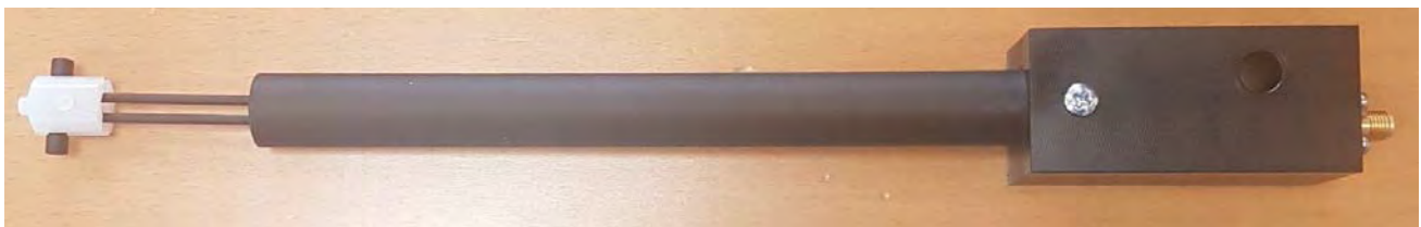
Figure 1 – MVG COMOSAR Validation Dipole
