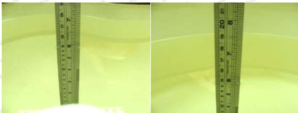
Photo of Liquid Height for Head SAR
