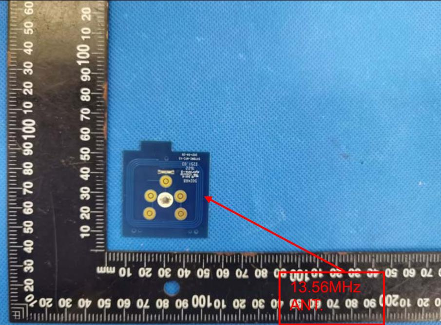
A photograph of a blue PCB (Printed Circuit Board) with a central component and four circular pads. A red arrow points from the text '13.56MHz ANT.' to one of the circular pads. The PCB is placed on a blue textured surface. A black ruler is positioned horizontally below the PCB, with markings in millimeters from 0 to 100. A red rectangular box highlights the text '13.56MHz ANT.' on the ruler. |                             |
