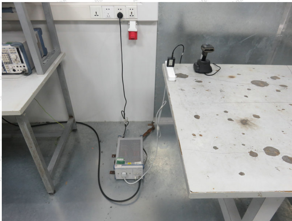
Photo of Conducted Emission Measurement
