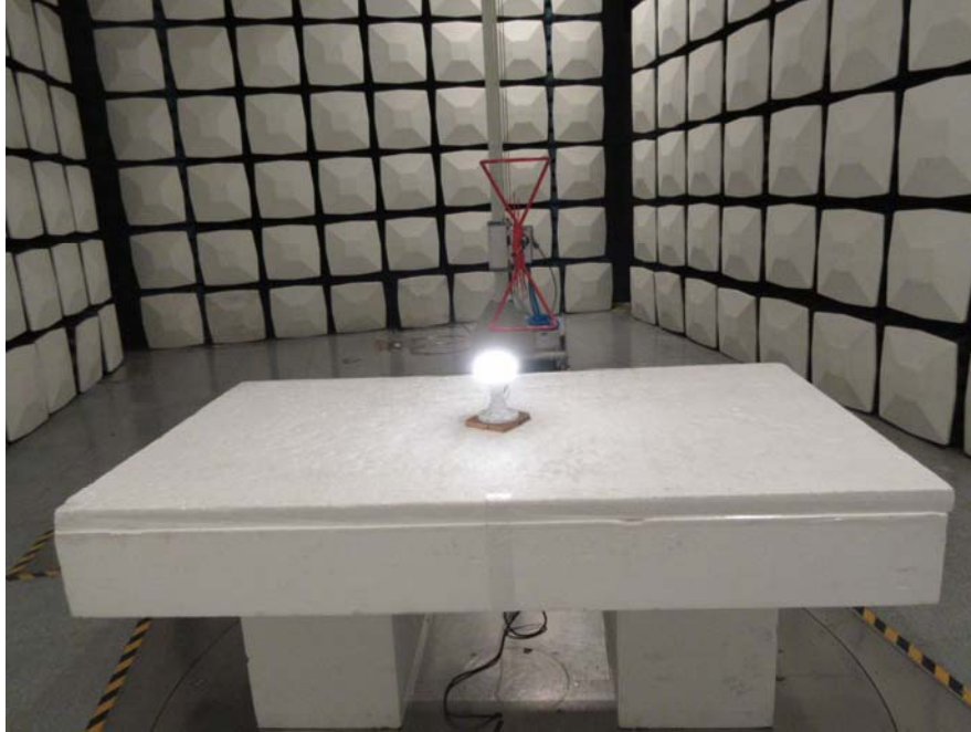
Radiated Emission View (Below 1 GHz)
