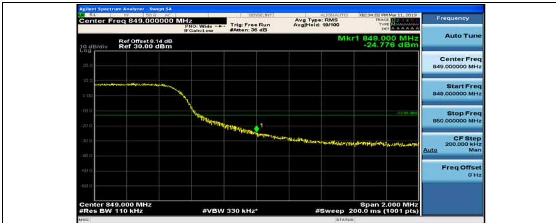
Channel Bandwidth: 10 MHz_HCH_QPSK_50RB#0
