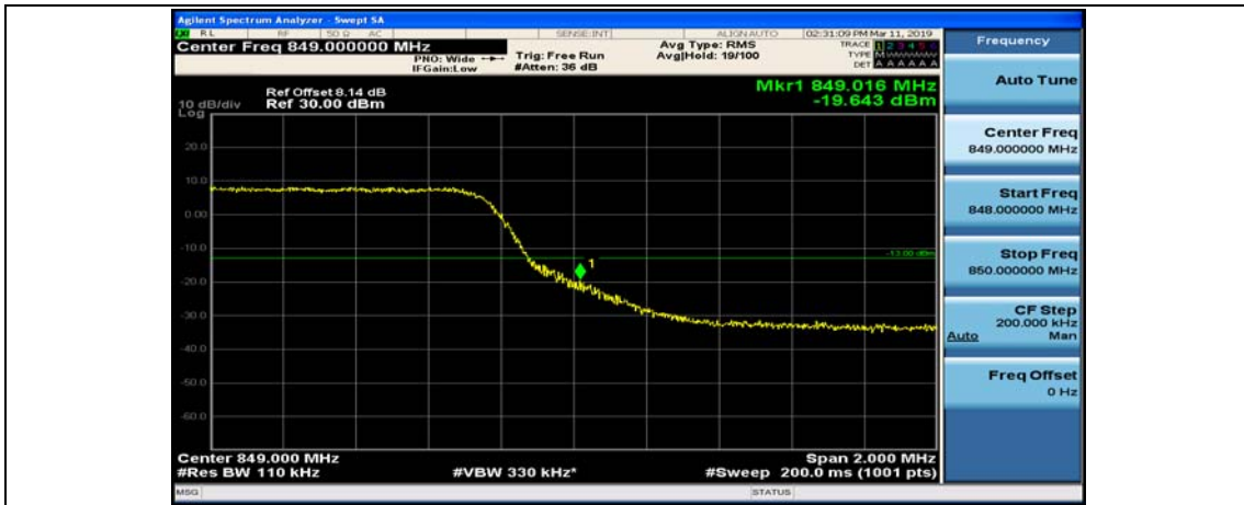
(Channel Bandwidth: 5 MHz)_LCH_16QAM_1RB#0
