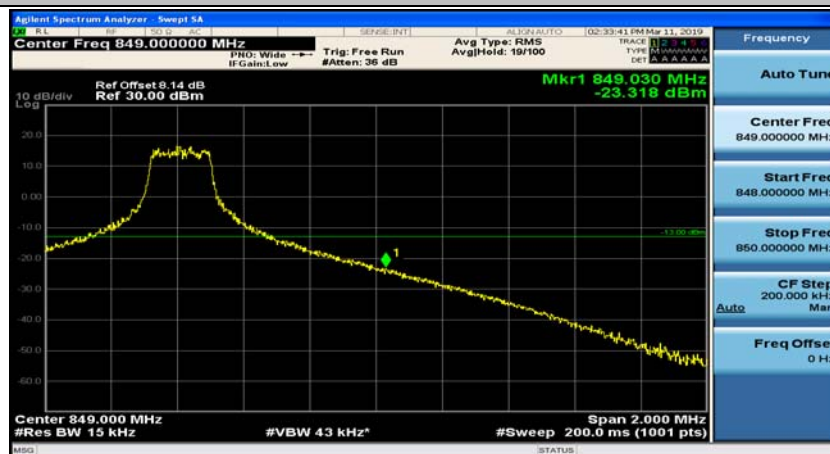
Channel Bandwidth: 10 MHz_HCH_16QAM_25RB#0
