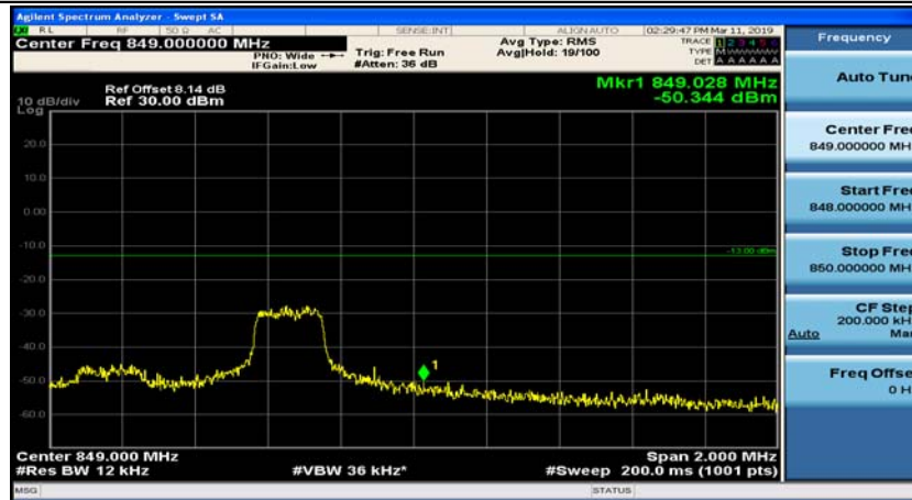
(Channel Bandwidth: 5 MHz)_HCH_QPSK_1RB#12
