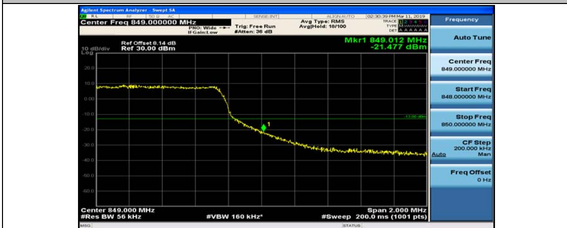
(Channel Bandwidth: 5 MHz)_HCH_QPSK_25RB#0
