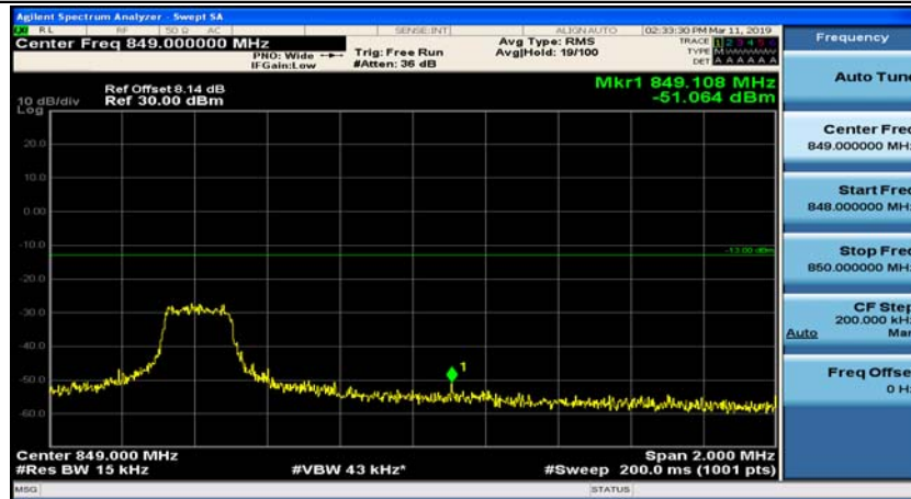
Channel Bandwidth: 10 MHz_HCH_16QAM_1RB#24
