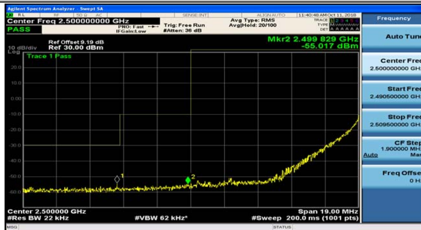
(Channel Bandwidth:20 MHz)_LCH_QPSK_1RB#99
