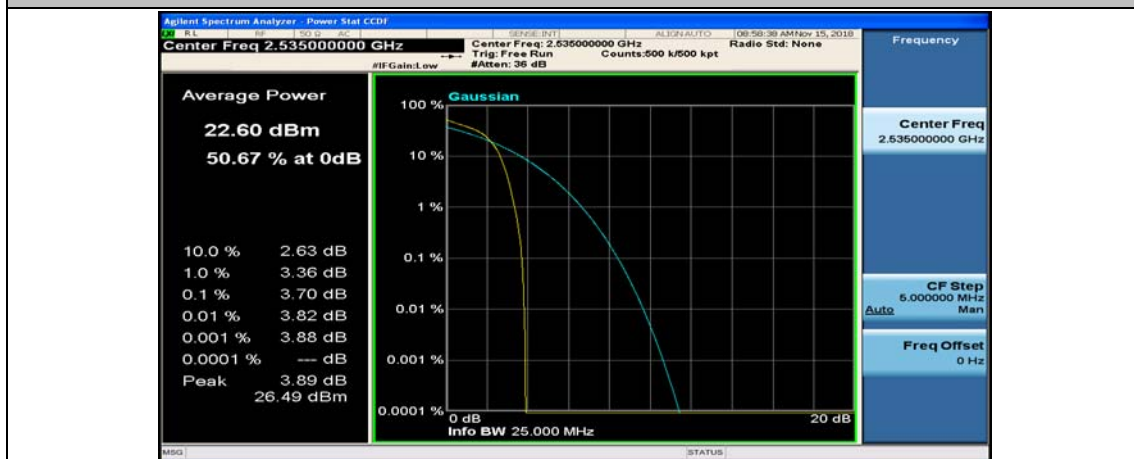
Channel Bandwidth: 10 MHz_MCH_16QAM_1RB#49
