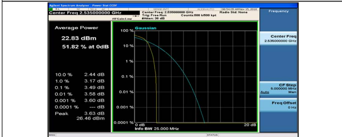
(Channel Bandwidth: 5 MHz)_MCH_16QAM_1RB#24
