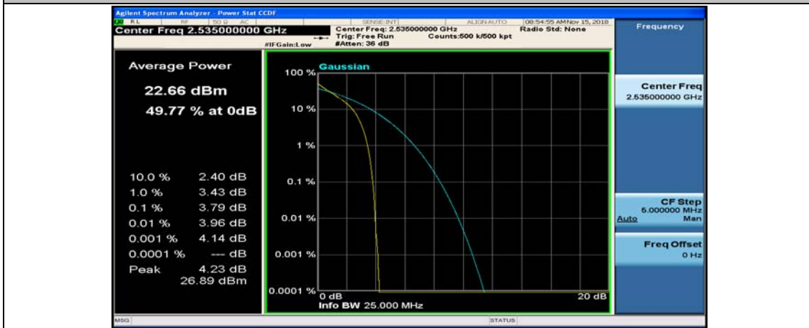
(Channel Bandwidth: 5 MHz)_MCH_QPSK_25RB#0
