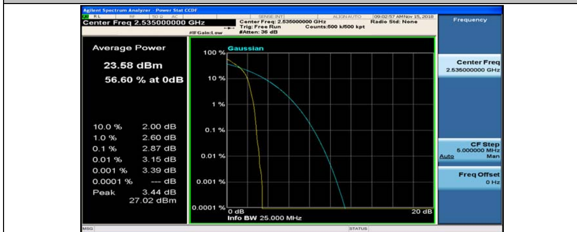
(Channel Bandwidth:15 MHz)_MCH_QPSK_1RB#37
