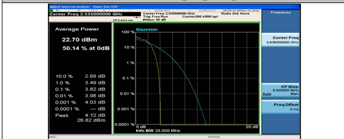
Channel Bandwidth: 10 MHz_MCH_16QAM_1RB#24
