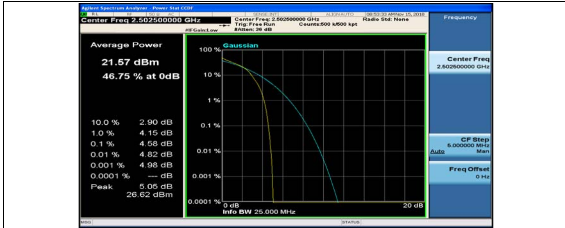
(Channel Bandwidth: 5 MHz)_MCH_16QAM_1RB#0
