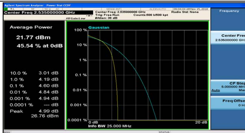
(Channel Bandwidth:15 MHz)_MCH_16QAM_37RB#38
