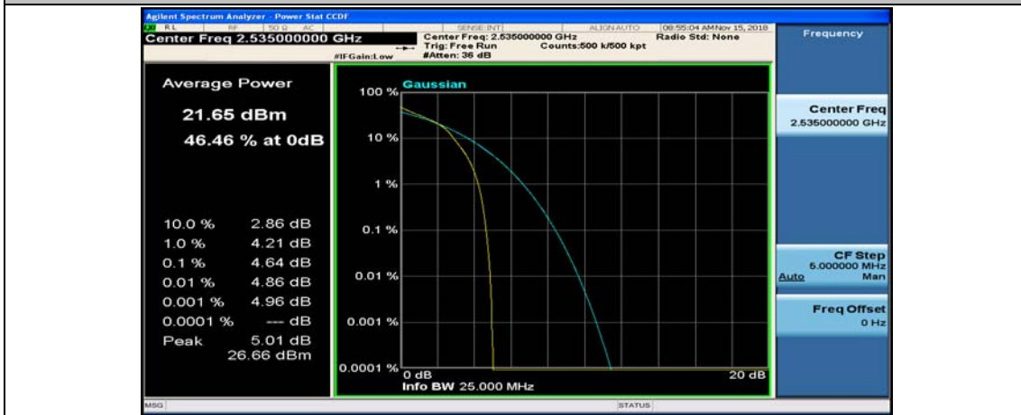
(Channel Bandwidth: 5 MHz)_MCH_16QAM_25RB#0
