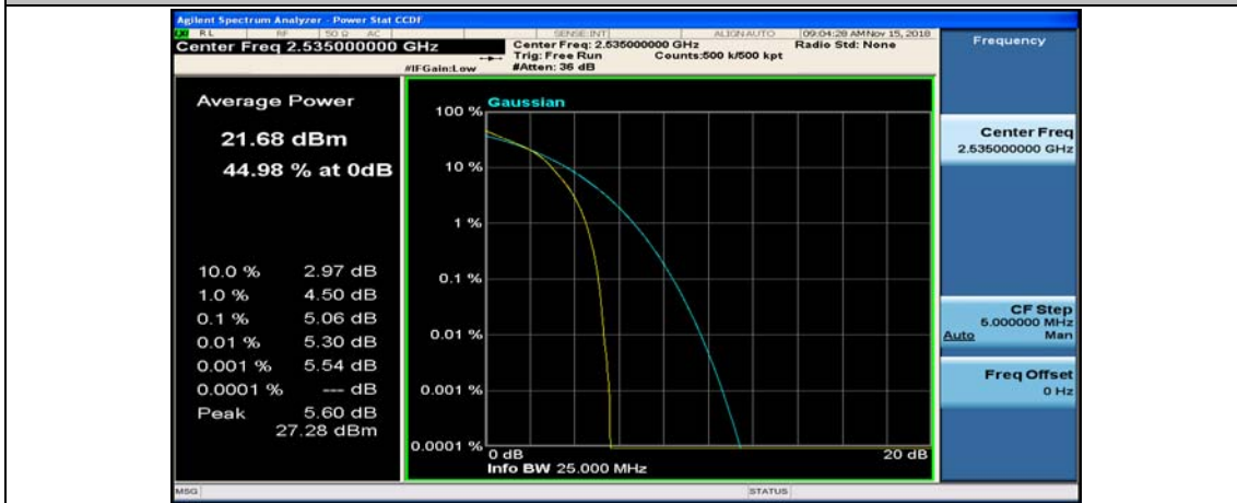
(Channel Bandwidth:15 MHz)_MCH_16QAM_75RB#0
