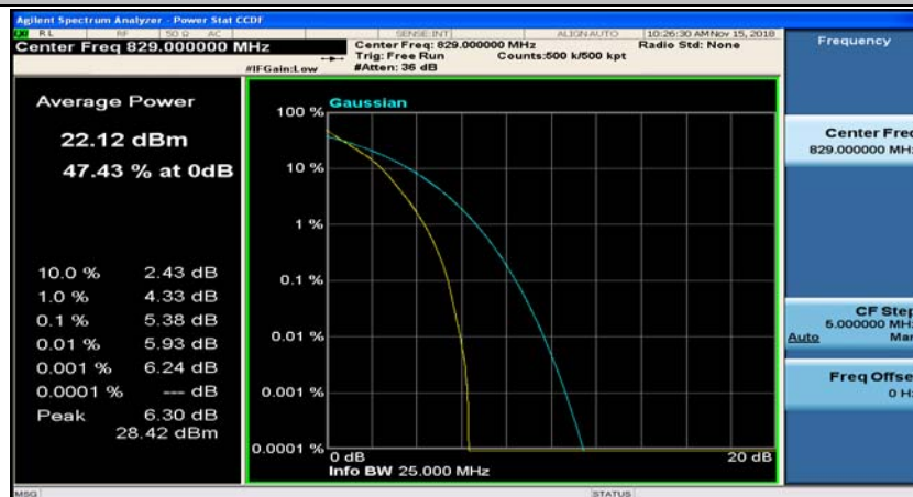
Channel Bandwidth: 10 MHz_LCH_QPSK_50RB#0
