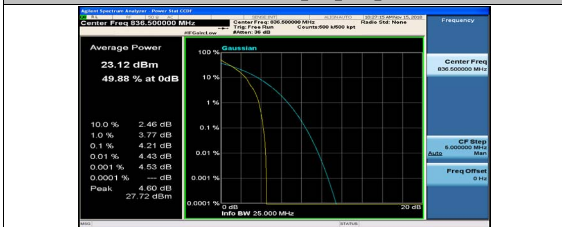
Channel Bandwidth: 10 MHz_MCH_QPSK_1RB#24
