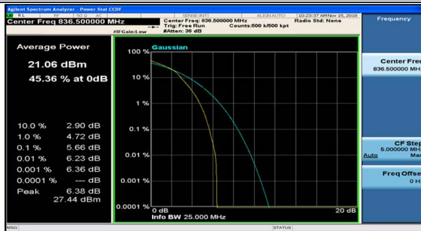
(Channel Bandwidth: 5 MHz)_MCH_16QAM_12RB#6
