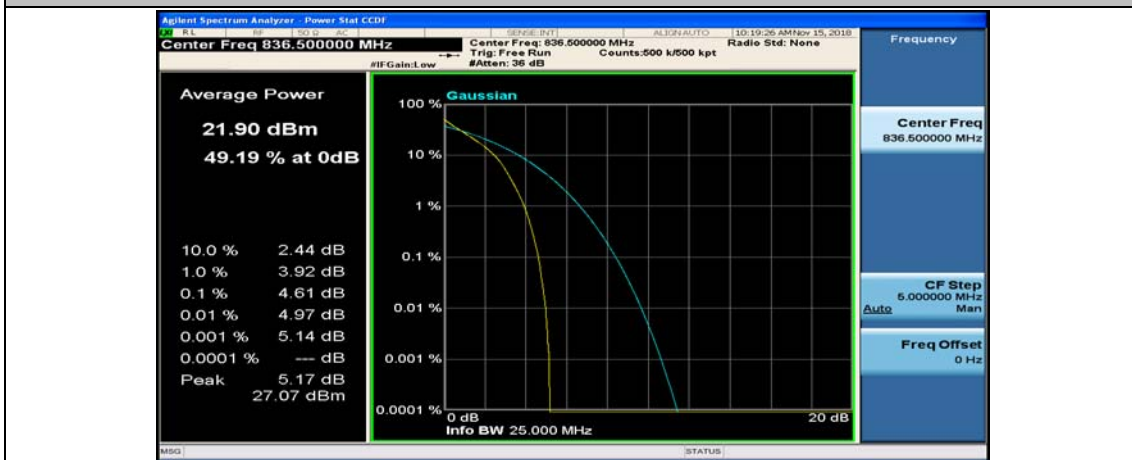
(Channel Bandwidth: 3 MHz)_MCH_QPSK_15RB#0
