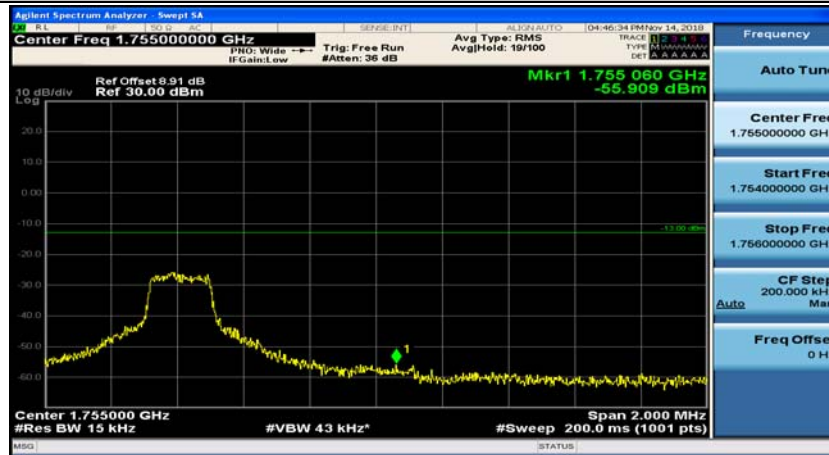
Channel Bandwidth: 10 MHz_HCH_16QAM_1RB#24
