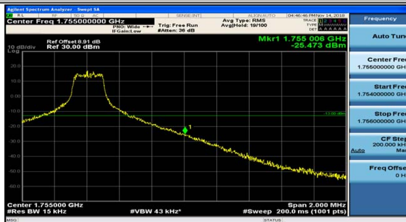
Channel Bandwidth: 10 MHz_HCH_16QAM_25RB#0
