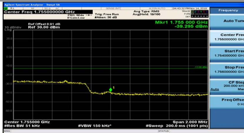
(Channel Bandwidth: 5 MHz)_HCH_QPSK_12RB#6
