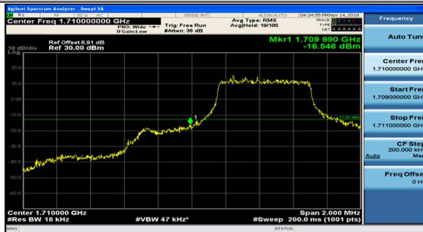
(Channel Bandwidth: 1.4 MHz)_LCH_QPSK_3RB#2
