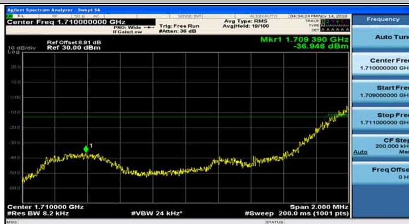
(Channel Bandwidth: 1.4 MHz)_LCH_QPSK_1RB#5
