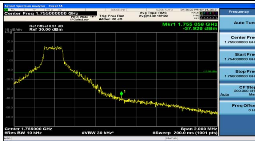
(Channel Bandwidth: 1.4 MHz)_HCH_16QAM_1RB#5
