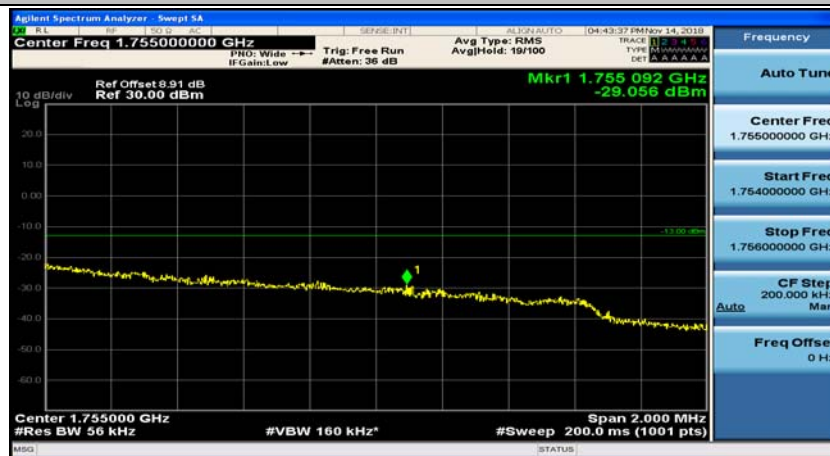
(Channel Bandwidth: 5 MHz)_HCH_QPSK_12RB#13
