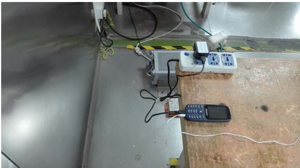
Conducted Emissions - Side View
