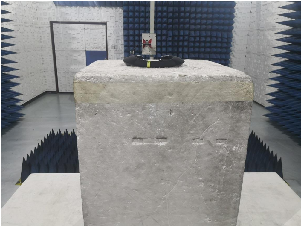
RADIATED EMISSION TEST SETUP ABOVE 1GHz
