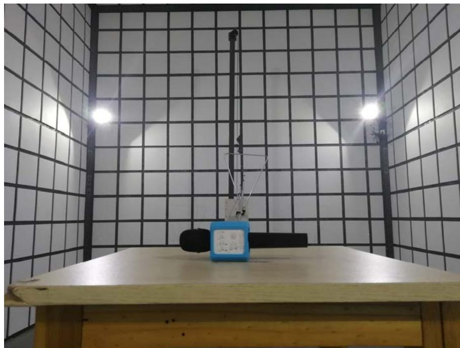
**Radiation Emission Test Setup (Above 1GHz)**
