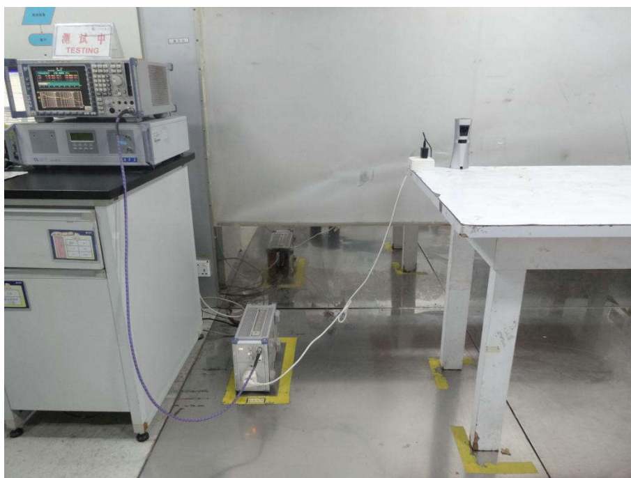
Conducted Emissions Test Setup
