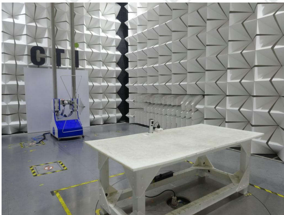
Radiated spurious emission Test Setup-2(30MHz-1GHz)
