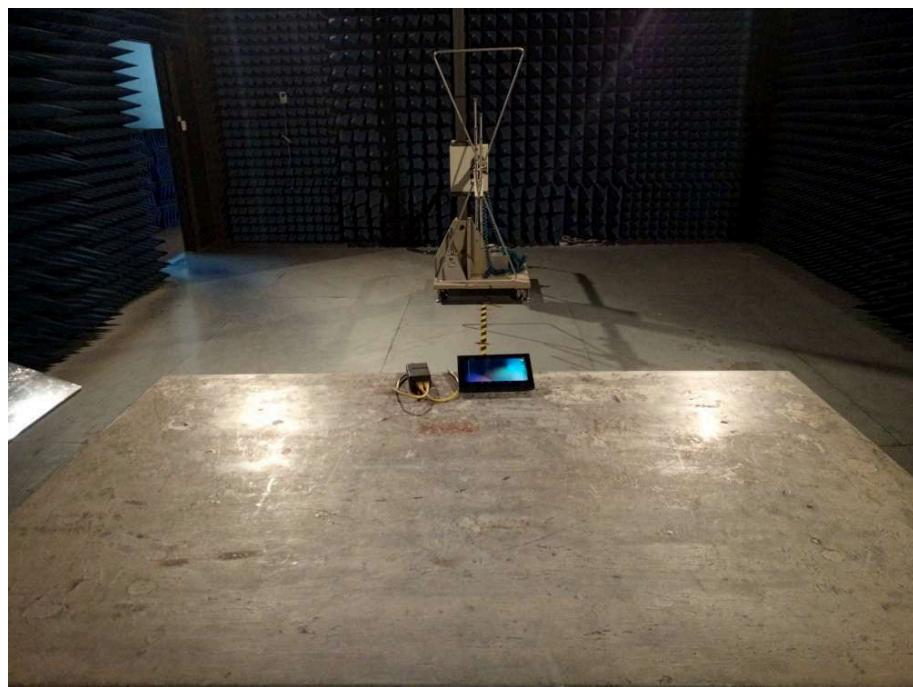
**Radiated Emission Test View 2**
