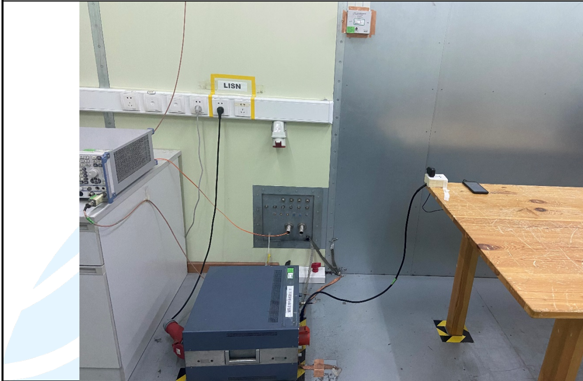
Conducted Emission Test Setup
