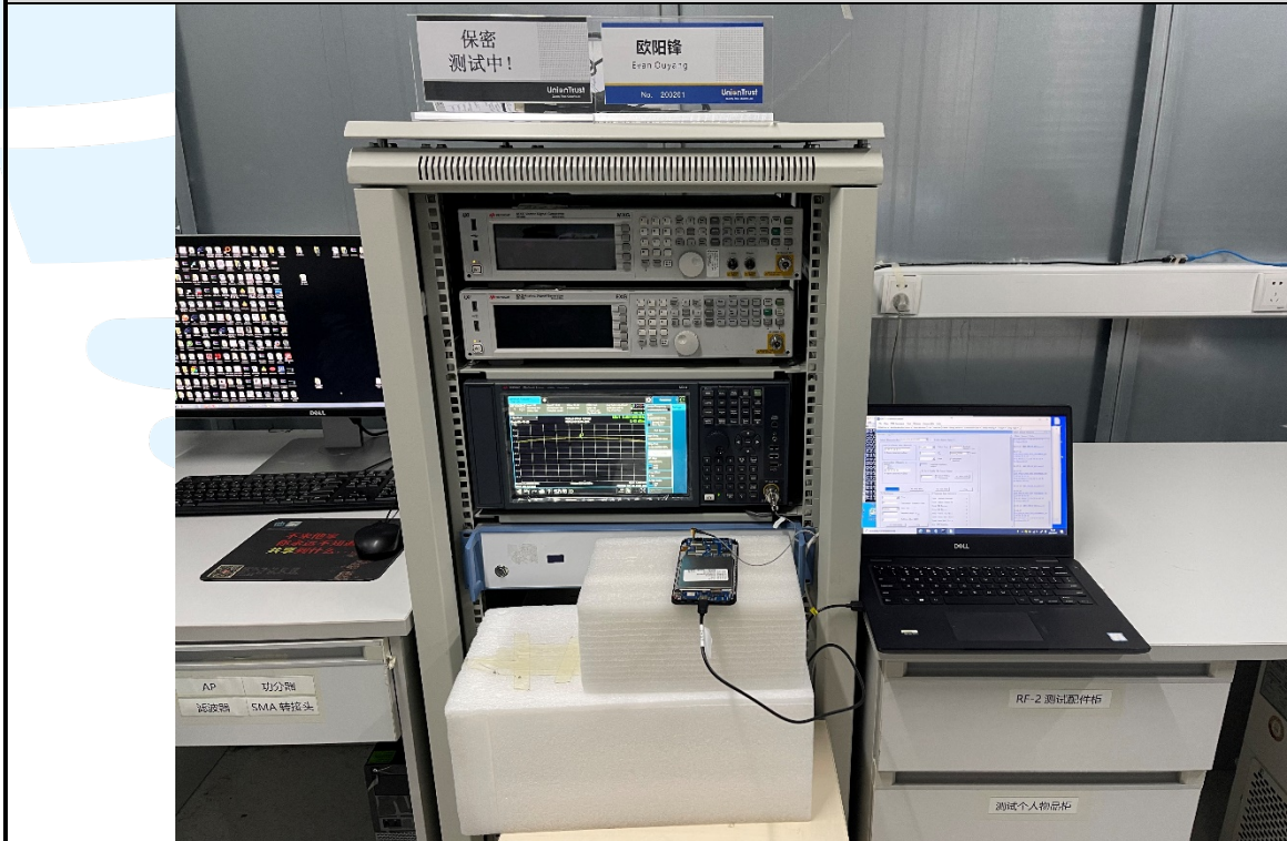
RF Conducted Test Setup
