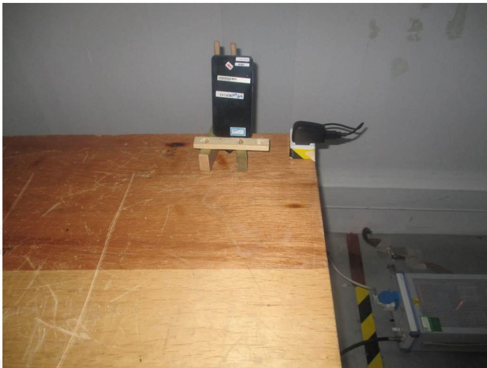
Power Line Conducted Emissions
