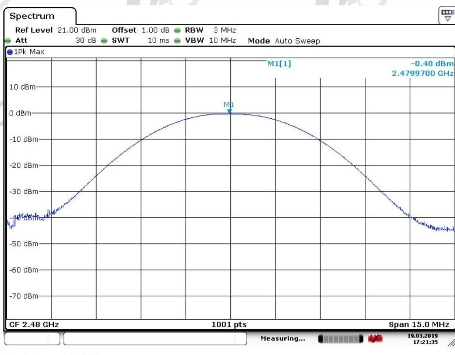
**DTS (6 dB) Bandwidth & 99% Occupied Bandwidth****Test Results**
