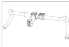
Step 2: Secure the mount with the rubber band.
