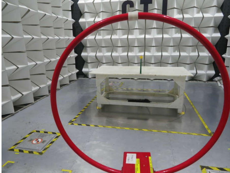
Radiated spurious emission Test Setup-1(Below 30MHz)
