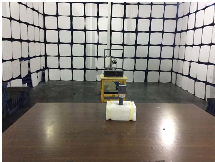
**Radiation Emission Test Setup (30MHz to 1GHz)**
