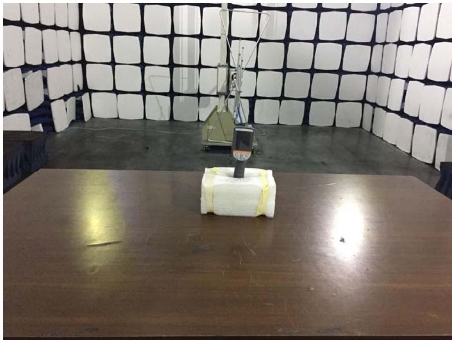
**Radiation Emission Test Setup (Above 1GHz)**
