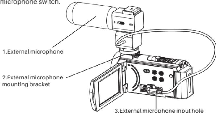
**!** Notice : The output impedance of external microphone is  $0.2K\Omega \sim 2.2K\Omega$  , Because each external microphone parameter is different, the specific effect is selected after actual adaptation.
