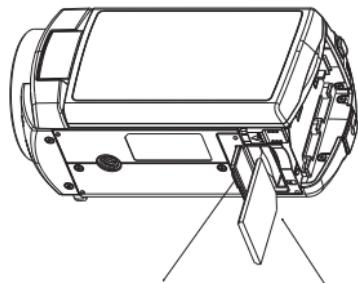
1.Open the memory card door (Toggle outside to open the memory card door, flip inside to close the memory card door)
