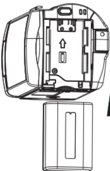
1. Install battery into the battery compartment according to this direction.
