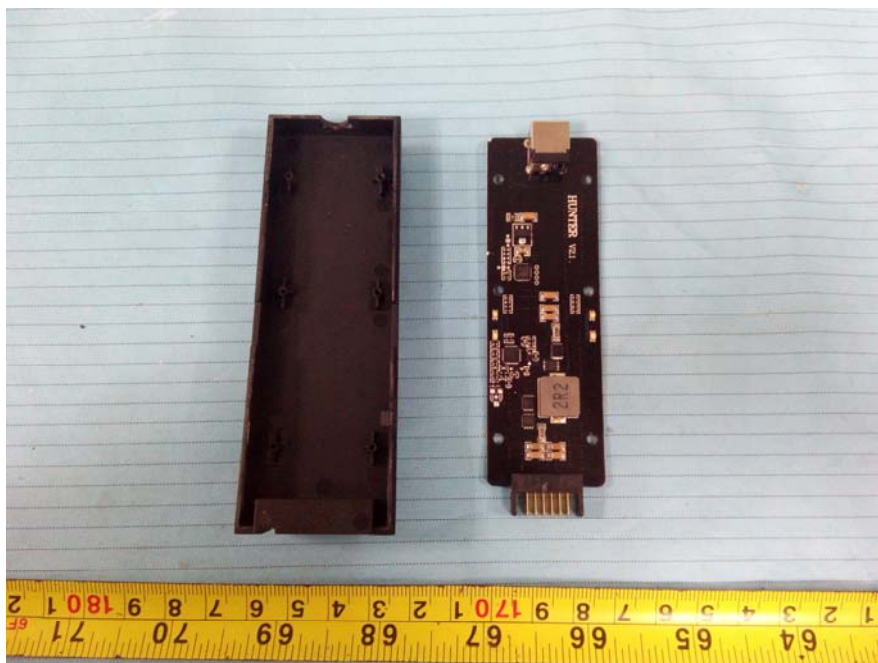
EUT – Cover off View 2 (Battery Charger)
