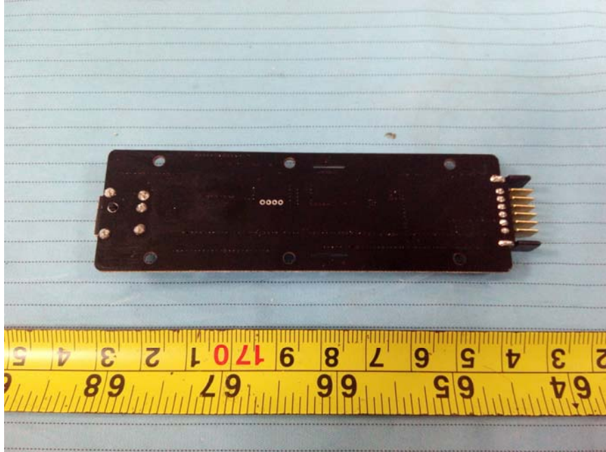
EUT – Main Board Bottom View (Battery Charger)
